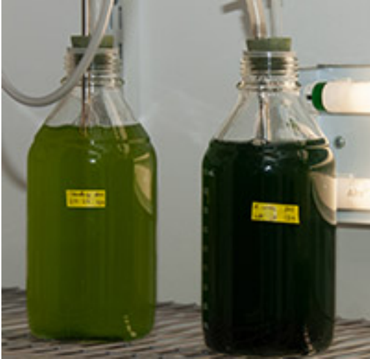
Green algae (on the left) and cyanobacteria (on the right) cultures being cultivated in the bottles use much more water than the algae grown as biofilms in the image above.
